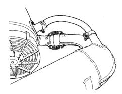
Ensure that the forced flow system is well aligned and tightened.
