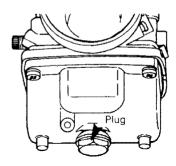
Re-install plug and connect fuel line.
