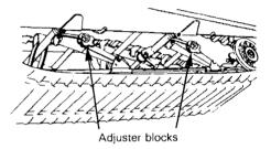
CAUTION: Always turn the left side adjuster blocks in a clockwise direction, the right side blocks in a counter-clockwise direction. Left and right adjuster blocks of each adjustment must always be set at the same elevation.
