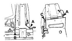
WARNING: At the removal or installation of the belt guard front retaining pin be careful not to burn yourself on the exhaust system.
