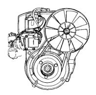
If the belt seems damaged or if tension is incorrect, contact your dealer immediately.
