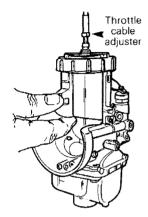
WARNING: It is important that the throttle slide adjustment be performed to ensure proper functioning of throttle mechanism.
